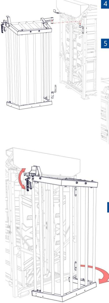
Lift the front cage and lower onto mech yoke...place onto top hinge (fitted to crush) to act as temporary hang support.
