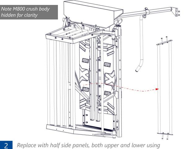
Replace with half side panels, both upper and lower using corresponding fitting holes.
