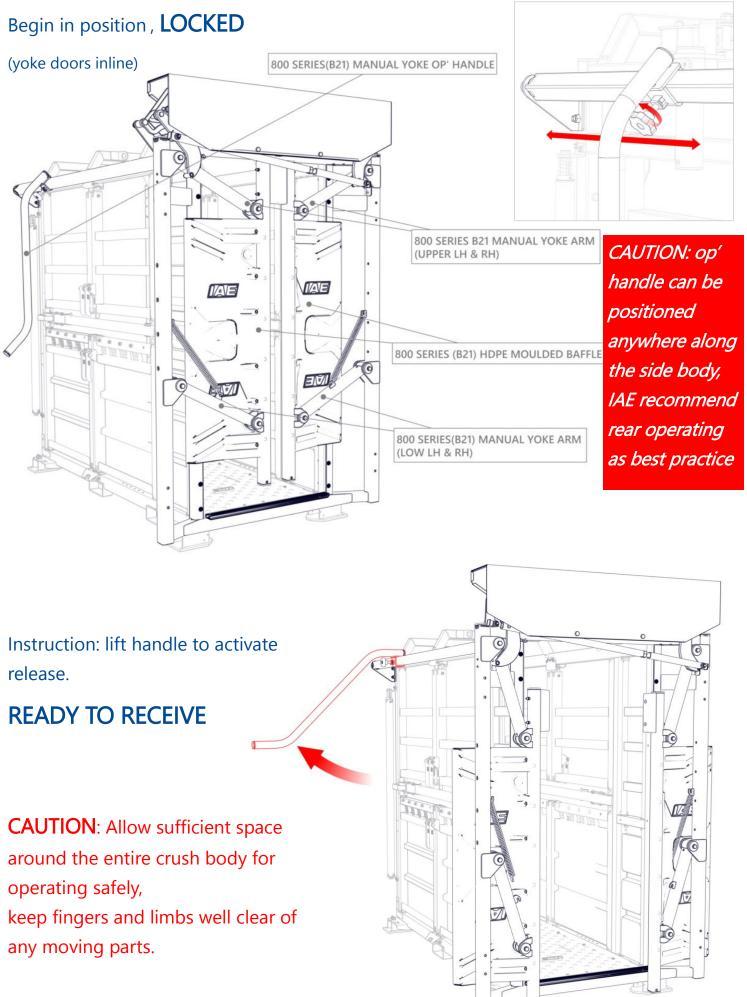
Instruction: allow animal to enter the chute, at the point when it's head and neck are positioned past the yoke doors, the operator can activate the yoke by lowering the operating handle.
