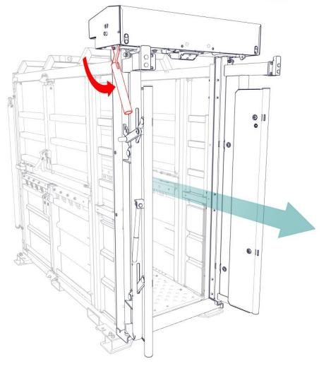
Instruction: push on yoke door to activate the auto yoke, making both doors drop back (angled into the chute).
