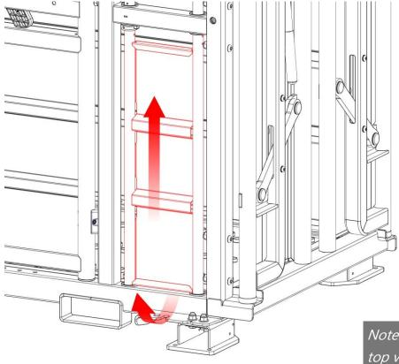
Instruction: lift (so tube end is free from bushes) and lift away to fully remove the panel.
