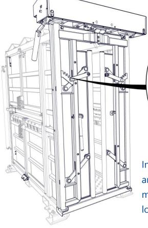
Instructions: lift the handle attached to the link arm to release from its original locking place. move up or down the 'hair comb like' slanted locking plate as required.
