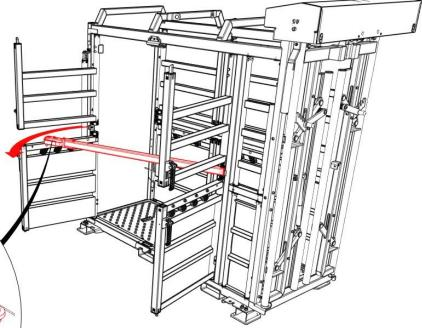
Option to reverse the side rail (situating the side rail operating handle to lock into the front end main body pillar, adjacent to vet access)
